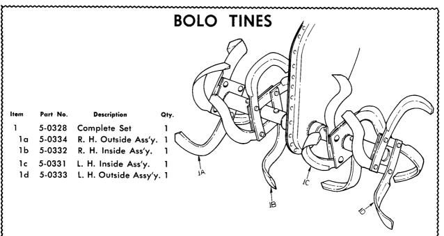
THE TINE BLADES ARE MADE FROM HEAT TREATED FORGED STEEL AND ARE SELF SHARPENING. IT HAS A TILLING WIDTH OF 26 INCHES. THESE TINES ARE RECOMMENDED FOR NORMAL CULTIVATION AND MULCHING JOBS.
