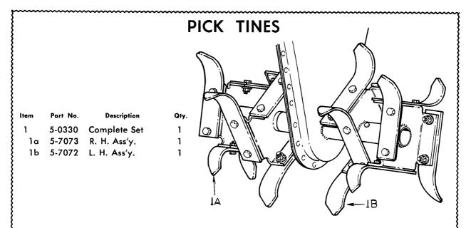
THIS SET OF TINES IS RECOMMENDED FOR USE IN THE TOUGH-EST SOILS, SUCH AS ROCKY GROUND AND HARD CLAY. THE PICK TINE WILL WORK WHEN OTHERS WILL NOT. IT HAS 16 RUGGED PICK POINTS FOR BETTER PENETRATION AND A TILLING WIDTH OF 16 INCHES.
