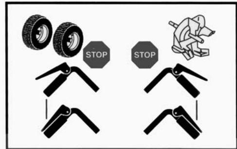
**DEADMAN CONTROLS.** Depress to engage. Release to disengage/stop. Left control – wheel drive. Right control – auger/impeller.
