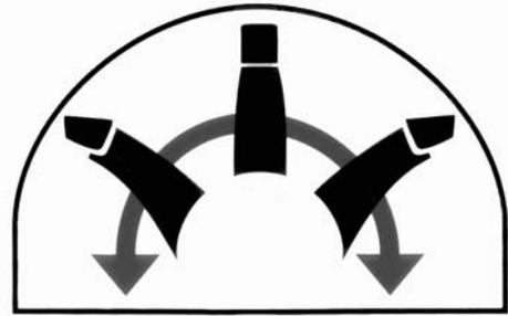
**DISCHARGE CHUTE.** Rotate control to discharge snow in desired direction.
