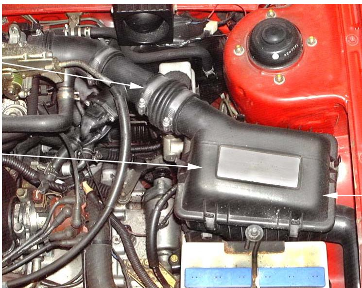
**3.** Remove the air box base from the inner wing by removing the 3 securing screws located inside of the air box base.
