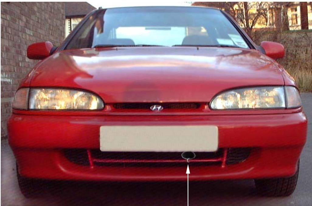
Pierce / Drill a 3mm hole in the end of the flexi cold air hose and feed the hose to the lower grille. Secure the end of the hose to the grille using a plastic tie supplied. It may be necessary to ovalise the end of the hose so that it will fit in the grille.
