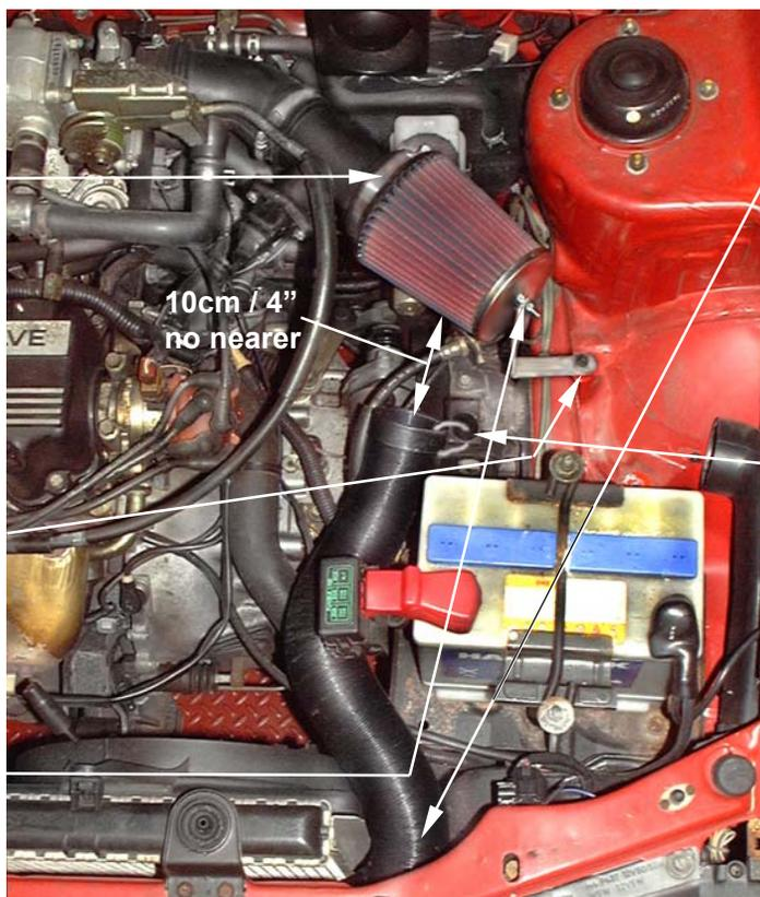
**4.** Carefully lengthen the flexi cold air hose to approx. 76cm / 30" and feed it down past the side of the radiator to the front lower grille.
