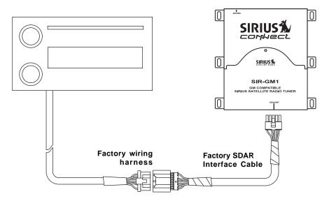
Remove the Factory XM Tuner and connect the SDAR Interface Cable
