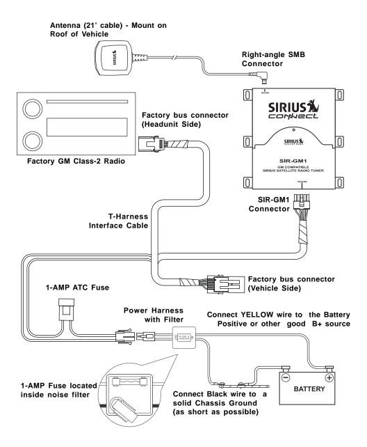
NOTE: If your vehicle is equipped with a factory satellite radio tuner and you are using the included 'T-harness interface cable' for installation, you must disconnect the factory satellite radio tuner at the tuner box. Otherwise, operational errors will occur while using the SIR-GM1.
