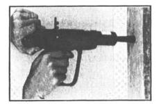
Depress the tool firmly against the work surface using both hands. Make certain you hold the tool perpendicular to the work. The tool is now in the firing position, if you have followed ALL safety precautions, pull the trigger.
