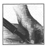
Insert the fastener into the nose piece of tool, head or threaded stud end first. Push fastener until the pointed end is even with the face of the nose piece.
