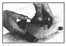
3. Remove the nose piece from the barrel. Inspect the piston buffer for damage.
