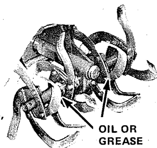
CLUTCH LEVER PIVOT POINTS, TINE HUBS AND TINE SHAFT, HANDLE SWIVEL KNOB ROD
