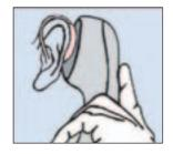
The telecoil mode is intended for telephone use. In the telecoil mode, place the telephone receiver close to your hearing instrument for best reception. By trying various positions with the telephone receiver, you will discover what works best for you.
