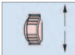
Rotate the wheel upwards to increase volume. Rotate it down to decrease volume.
