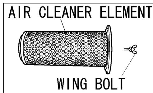
Loosen the wing bolts in the air cleaner and remove the air element.
