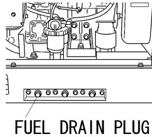
Unscrew the fuel drain plug.
