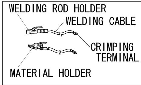
Connect the welding cables to the output terminals per the table below.
