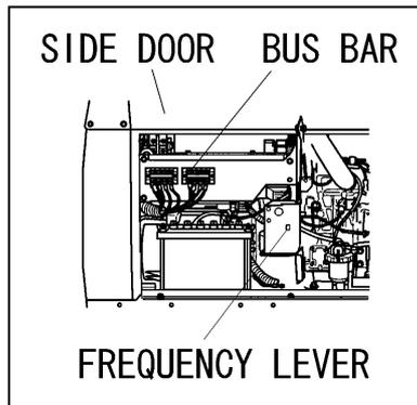
Turn the selector switch and the metal bus bars to the other frequency as per the drawing.
