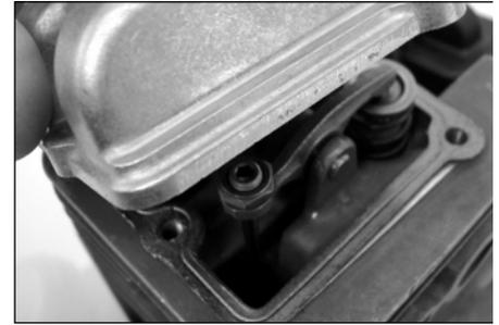
6. Turn engine over several times, and return to TDC-compression. Recheck with proper feeler gauge to make sure clearance adjustment did not change as a result of tightening the locknut. Readjust as necessary.
