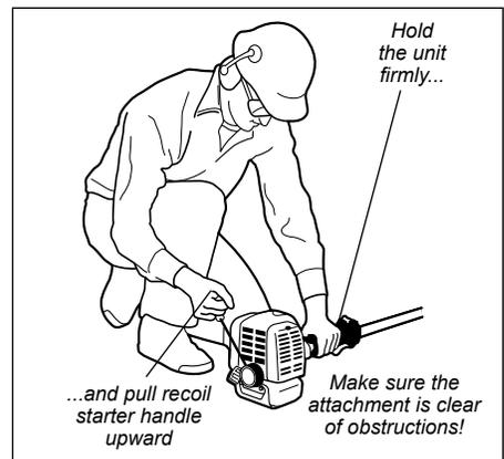
6. When the engine starts, slowly move the choke lever to the “OPEN” position. (If the engine stops after the initial start, close the choke and restart.)
