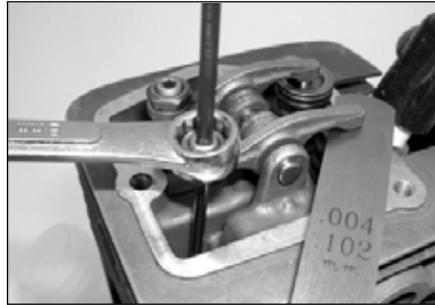
2. Loosen adjuster locknut so that the 2.5 mm Allen socket head adjustment screw can turn freely.
