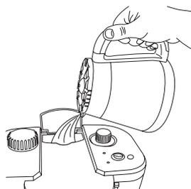
**4a** - Fill the reservoir to the 1.2L Max fill line as indicated on the water level gauge
