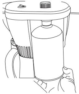
**2a** - For use with Butane open the fuel compartment remove the included brass butane adaptor, thread the adaptor onto a butane canister and insert the butane canister and adaptor and attach by pushing up and turning counter clockwise.
