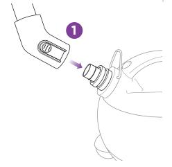
Use the steam bonnet on the nozzle to prevent water drops from being left on the garment and to improve performance.
