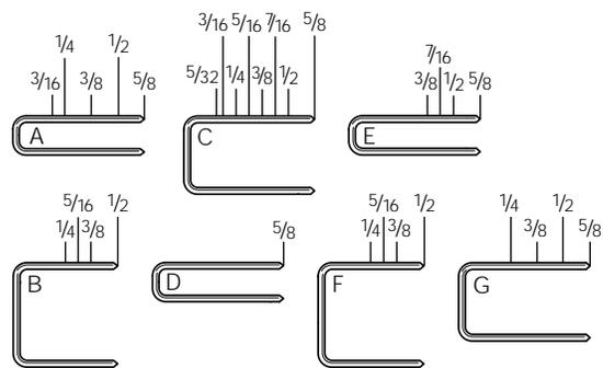
Available Crown Widths 3/16", 3/8", 1/2". 22 Gauge Staples. 5/32" - 5/8" Lengths. Capacity 110-185.
