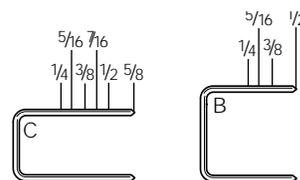
Available Crown Widths 3/16", 1/2". 22 Gauge Staples. 1/4" - 5/8" Lengths. Capacity 180.
