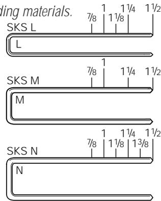
Available Crown Widths 1/4", 3/8", 1/2", 5/8", 7/8", 1", 1 1/4", 1 1/2" Lengths. Capacity 145-158.
