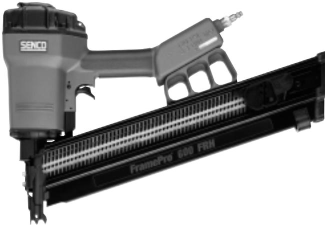
The FramePro® Full Round Head Nailers are the result of our award winning, feature loaded clipped head nailers now designed for Full Round Head nails. The FramePro® 600/650 FRH nailers feature an aggressive toenail safety, rugged aluminum casting, power to drive full round head nails from 2" to 3½" in 5 gauges (.113-.162) and an in-line magazine for superior balance and line of sight. All this and more for the Pro. Senco tools. Hard Work. Bring it On!
