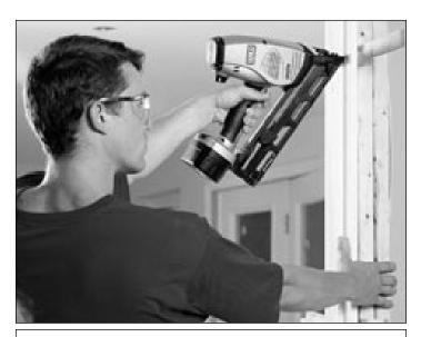
\* "Restrictive Trigger" activated tools are used for applications where precision nail or staple placement is desired. You must first depress the safety element where you want to drive a nail or staple and then pull the trigger. After each nail or staple is driven, completely release the trigger and lift the tool off the work surface.
