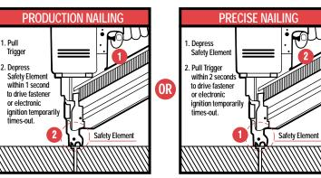
If a fastener isn't driven within the allotted time, ThinkTrac's electronic ignition temporarily "times-out". Before a fastener can be driven, the trigger must be released and the safety element lifted off the work surface—a habit that promotes safety.
