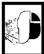
ARC RAYS CAN INJURE EYES AND BURN SKIN! To reduce risk of injury from arc rays, read, understand, and follow the following safety instructions. In addition, make certain that anyone else that uses this cutting equipment, or is a bystander in the cutting area, understands and follows these safety instructions as well.
