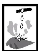
PLASMA ARC CUTTING CAN CAUSE SERIOUS BURNS FROM HOT SLAG OR MOLTEN METAL! To reduce risk of injury from serious burns caused by flying or dripping hot slag or molten metal, read understand and follow the following safety instructions. In addition, make certain that anyone else who uses this cutting equipment or a bystander in the cutting area understands and follows these safety instructions as well.
