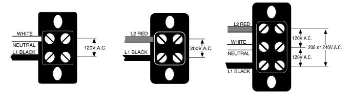
These brewers require 2-wire, grounded service rated 120 or 200 volts ac or 3-wire, grounded service rated 120/208 or 120/240 volts ac, 20 amp, single phase, 60 Hz. Refer to the product's data plate above the dilution nozzle for actual voltage of your particular brewer model.
