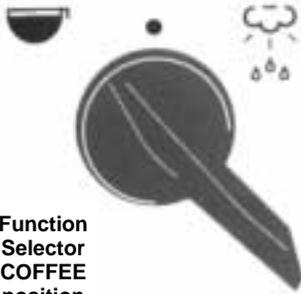
7. When the Green "GO" Light illuminates, flip the Function Selector (on the side of the machine) to "COFFEE CUP".
