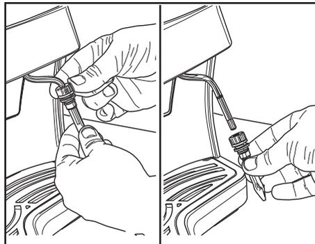
Loosen the ring nut and remove the internal part of the pannarello. After washing it thoroughly, reassemble it taking care to position it as shown in the figure.
