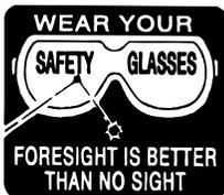
The operation of any reciprocating saw can result in foreign objects being thrown into your eyes, which can result in severe eye damage. Before beginning power tool operation, always wear safety goggles or safety glasses with side shields and a full face shield when needed. We recommend Wide Vision Safety Mask for use over eyeglasses or standard safety glasses with side shields.
