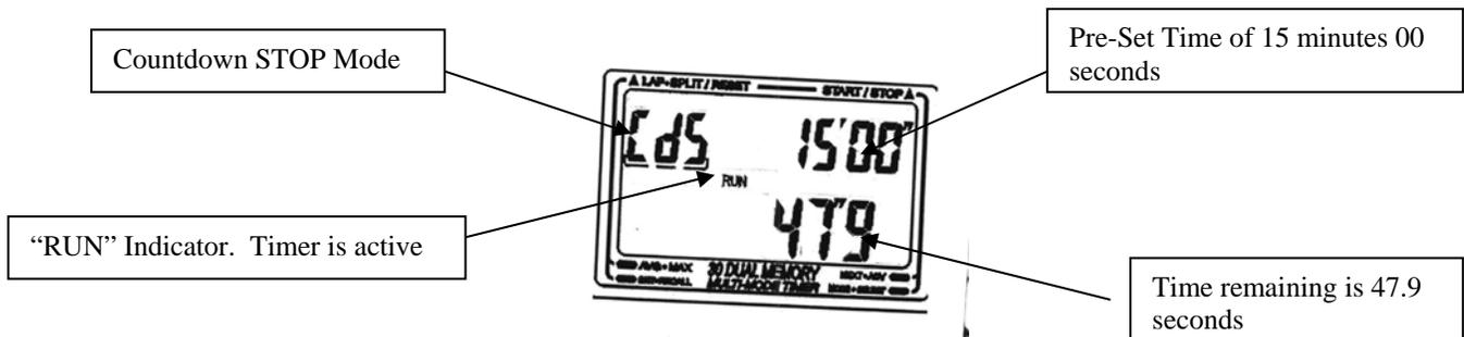
“Time Out”. You may stop and restart the CDT by pressing “A”. While stopped, the “STOP” indicator will appear. You may restart the timer by pressing “A” or reset to the original preset time by pressing “B”.
