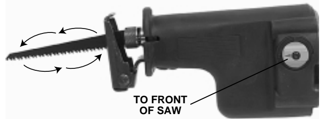
Figure 2 – Saw motion when lever points to left
