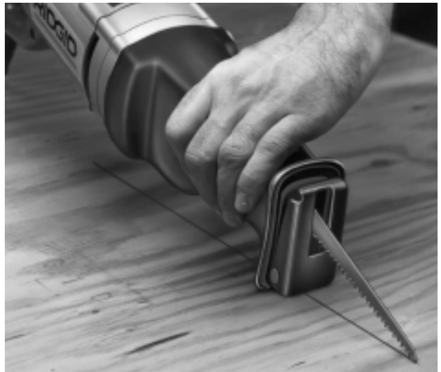
Figure 6 – Starting plunge cut
