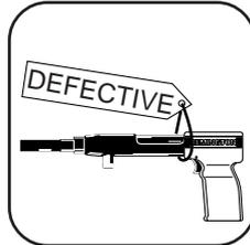
2. **ALWAYS** inspect to make sure the tool is working properly. If the tool does not work properly, remove from service and tag **DEFECTIVE**. **DO NOT** use the tool again until it has been properly repaired.
