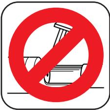
8. **NEVER** pry a power load out of the tool. Prying can discharge the load causing serious injury (see *Troubleshooting Guide*, page 16).
