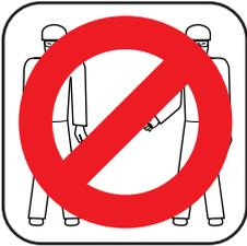
4. **NEVER** carry or pass a loaded powder actuated tool. **NEVER** point a powder actuated tool at anyone.
