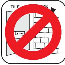
2. **NEVER** attempt to drive power fasteners into very hard or brittle materials including, but not limited to cast iron, glass, tile, stone, brick, or hardened steel. Materials of this type tend to shatter and create hazard from flying particles.
