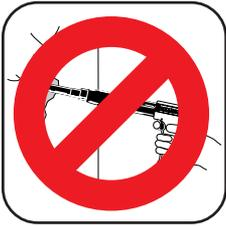
3. **NEVER** make fastenings in spalled or cracked areas.
