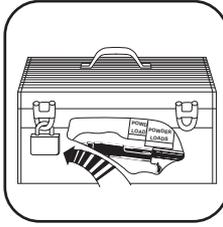
3. **ALWAYS** store **UNLOADED** powder actuated tool and power loads in a locked container. Keep power loads of different power levels in separate containers.
