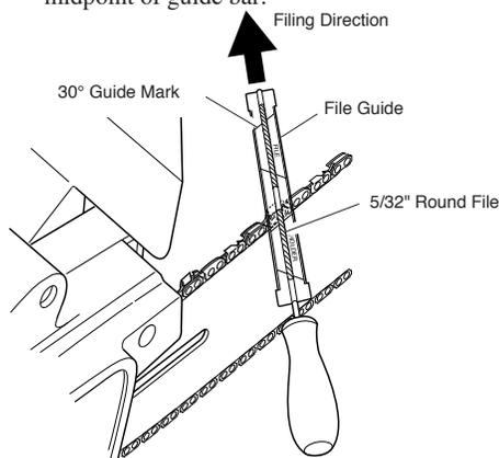
**Note:** This illustration shows file guide placement and filing direction for sharpening cutters on left side of chain.
