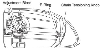
**Figure 6 - Turn Chain Tensioning Knob on Model 107625-02, 111174-01**
