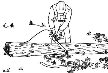
Figure 14 - Bucking Log With Entire Length On Ground
