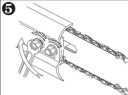
**5** Make sure chain moves freely around guide bar then tighten both nuts.
