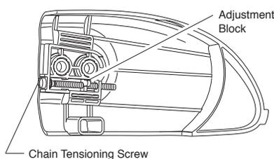
**Figure 5 - Turn Chain Tensioning Screw on Model 107624-02**
