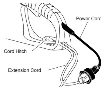
**Figure 9 - Looping Extension Cord over Cord Hitch**
