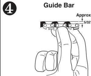
**4** Pull chain to check tension. Guide links should not come out of guide bar groove...
