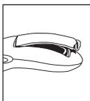
■ Insert the batteries so that the (+) and (-) marks on the batteries face the same marks inside the battery compartment. The BKT-1500 will not operate if batteries are inserted incorrectly.
