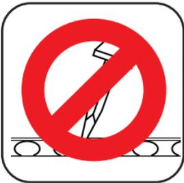
8. Never pry a power load out of the strip. Prying can discharge the load causing serious injury (See *Troubleshooting Guide*, page 26). Never attempt to reload used strips.
