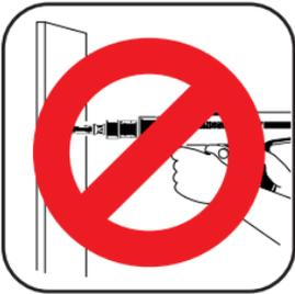
4. **NEVER** drive power fasteners into thin or easily penetrated materials unless it is backed by concrete or steel. When in doubt, such as when base material is concealed, conduct a Center Punch Test (See page 6). Check continually to avoid fastening into unsuitable material, especially in older buildings.
