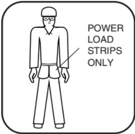
4. **NEVER** carry fasteners or other hard objects in the same pocket or container with power load strips.
