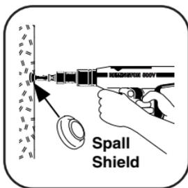
3. **ALWAYS** use the spall shield when driving directly into concrete or steel. Always wear goggles.
