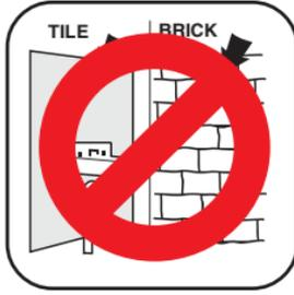
2. **NEVER** attempt to drive power fasteners into very hard or brittle materials including, but not limited to cast iron, glass, tile, stone, brick, or hardened steel. Materials of this type tend to shatter and create hazards from flying particles.
