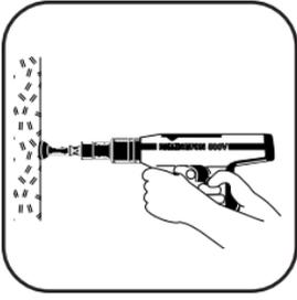
5. Squeeze trigger to set power fastener. Be sure to keep pressure on tool during this operation.
