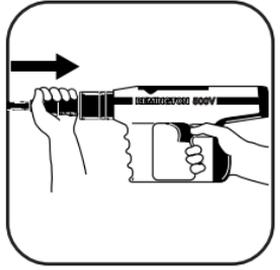
1. Grasp barrel assembly and slide forward rapidly until it stops. Push barrel assembly back into tool to the closed position. This sets piston into firing position.
