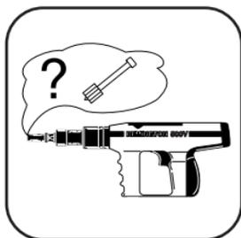
1. **ALWAYS** handle the tool as if it were loaded. Before starting work, check that the tool is unloaded and the muzzle is clear. **NEVER** load a tool unless it is going to be used.
