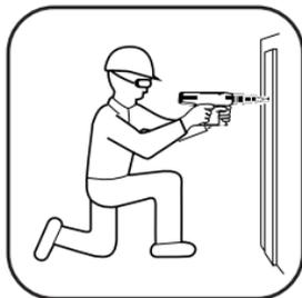
3. Operators and bystanders must **ALWAYS** wear goggles and hearing protection which meet or exceed the accepted standards for adequate protection in your country. In the USA, refer to ANSI standards. In Canada, refer to CSA standards.
