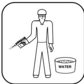
2. Should the tool fail to fire, hold the muzzle firmly against the work surface for 30 seconds. Release the trigger and remove pressure on the tool while holding the muzzle against the work surface. Again press the tool firmly against the work surface and pull the trigger. If the tool still fails to fire, hold the tool firmly against the work surface for another 30 seconds before advancing the power load strip. Use remaining loads in strip. Discard power load strip into water or oil.
