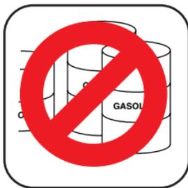
4. **NEVER** use a powder actuated tool in an explosive or flammable atmosphere or when non-sparking tools are required.
