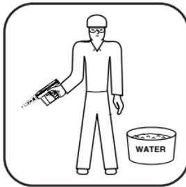
7. Should the tool fail to fire, hold the muzzle firmly against the work surface for 30 seconds. Release the trigger and remove pressure on the tool while holding the muzzle against the work surface. Again press the tool firmly against the work surface and pull the trigger. If the tool still fails to fire, hold the tool firmly against the work surface for another 30 seconds before advancing the power load strip. Use remaining loads in strip. Discard power load strip into water or oil.
