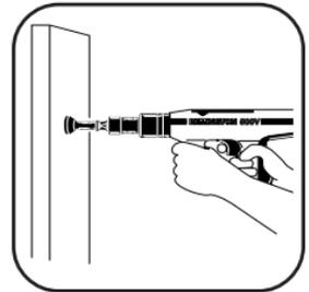
2. **NEVER** place your finger on the trigger until the tool's muzzle is against the work surface.
