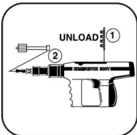
9. If work is interrupted for any reason, remove the power load strip before removing the power fastener.
