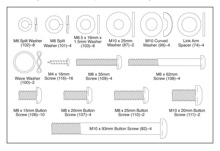
While another person lifts the front of the Frame (1), attach the Front Stabilizer (4) to the Frame with two M10 x 93mm Button Screws (82) and two M10 Curved Washers (99).
