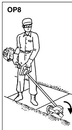
1. Always wear eye protection such as safety goggles. Never lean over the rotating cutting head. Rocks or other debris could be thrown into eyes and face and cause serious personal injury.
