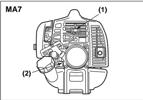
sure that the muffler is clean and free of wood chips, leaves, and other waste before use.
