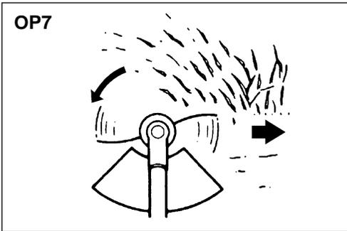
1. Hold the unit so the head is off the ground and is tilted about 20 degrees toward the sweep direction. (OP7)
