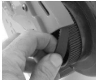
*Fig 19 & 20. Loosen the axle and push the wheel forward in the slots to loosen the belt as shown.*
