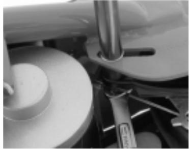
*Fig. 16. Loosen brake housing anchor and disconnect.*
