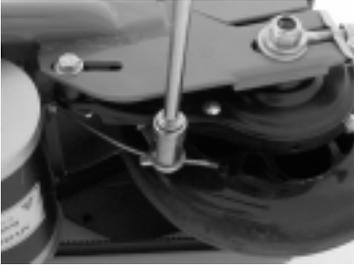
*Fig. 15. Loosen brake cable anchor and disconnect the cable.*
