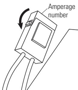
**4** Close the fuse box. Replace seat/storage compartment with the four (4) Phillips head screws.
