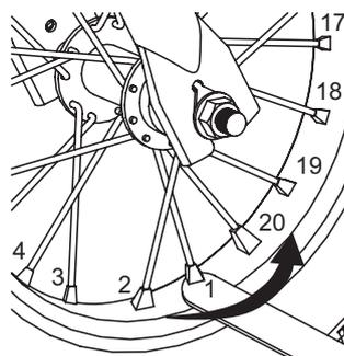
**2** Start with spoke closest to tire valve and tighten each nipple. In sequence, exactly 1/4 to 1/2 turn. A single 1/4 to 1/2 turn may not be enough to bring the spokes into proper tension. Continue tightening all spokes no more than 1/2 turn in sequence until all spokes are tight.
