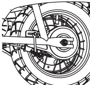
**2** With two 8mm wrenches, loosen brake housing anchor and disconnect. Keep the spacer and washers together
