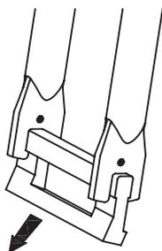
**1** Remove the packing material from the front fork.
