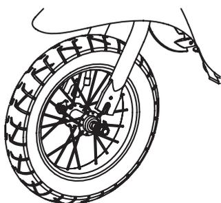
**2** Insert the wheel into the front fork with the lock washers on the outside of the fork.
