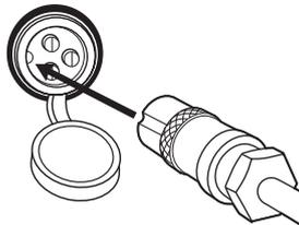
**1** Turn power **OFF** before charging. Plug the charger into the charger port.
