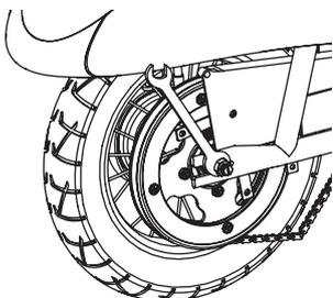
**4** With two 15mm wrenches, loosen the axle. Slide the wheel forward to loosen the chain and remove the wheel. Note the sequence of the hardware.
