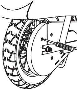
**1** With a Phillips screwdriver, remove the screws that secure the chain guard. Remove chain guard.
