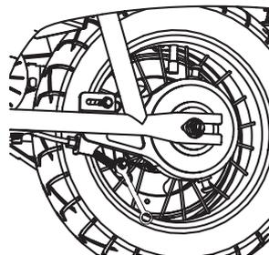
**3** With a 10mm wrench, loosen the brake cable anchor and disconnect the cable.
