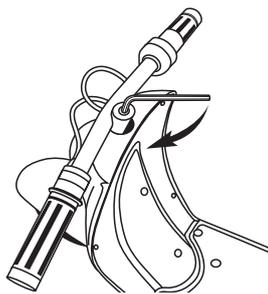
**2** Tighten down the hexagonal bolt with the 6mm hexagonal key wrench.
