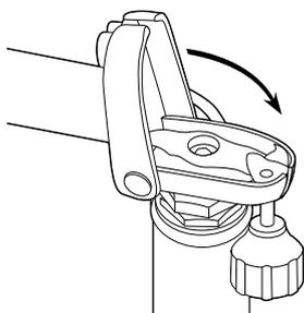
**5** Pivot the handlebar assembly upright.
