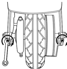
**3** Using a 10mm wrench, tighten the tension adjusters on the axle 1/8 to 1/4 turn to fine-tune the chain tension. Both adjusters must be tightened the exact same amount to maintain wheel alignment.
