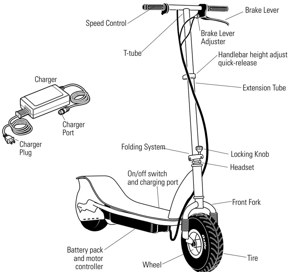
**WARNING:** DO NOT USE NON-RAZOR PRODUCTS WITH YOUR RAZOR ELECTRIC SCOOTER. The scooter has been built to certain Razor design specifications. The original equipment supplied at the time of sale was selected on the basis of its compatibility with the frame, fork and all other parts. Certain aftermarket products may or may not be compatible.
