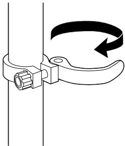
**1** Pull the quick-release lever outward.
