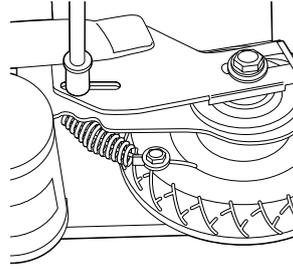
**12** Tighten the brake housing anchor securely. Test ride and check. Readjust as needed.
