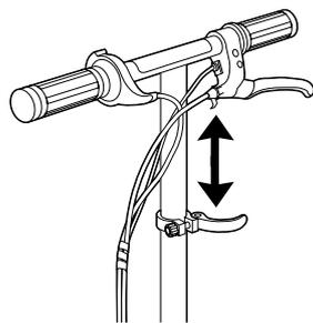
**2** Slide the T-tube to the desired position and secure by pushing the quick-release lever.
