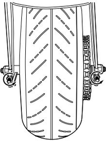
**4** With a 10mm wrench, loosen both axle adjusters an equal amount, about five turns.
