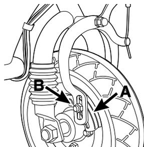
**2 (E100)** Inspect the brake pads (A) for proper alignment against the wheel or excess wear. To realign brake pads, loosen the fixing nut (B) and adjust the pad to contact the rim. Retighten and test the function, readjust as needed.
