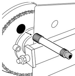
**3** Remove valve adapter immediately after inflating.
