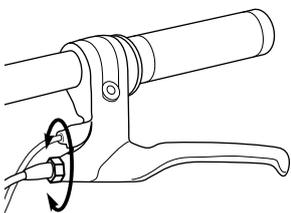
**1** To adjust the brake cable play, thread the brake lever adjuster in or out 1/4 to 1/2 turn until the desired brake adjustment is attained. Most adjustments are complete at this step. If brake still needs further adjustment, proceed to step 2.
