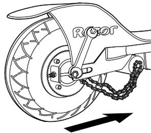
**5** With two 17mm wrenches, loosen the axle. Push the wheel forward in the slots to loosen the chain.
