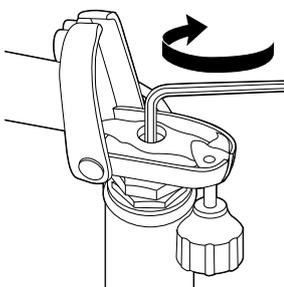
**4** Using a 6mm hexagonal key wrench, tighten the wedge by turning the bolt clockwise. The wedge is properly tightened when the handlebars cannot be twisted out of alignment with the front wheel.
