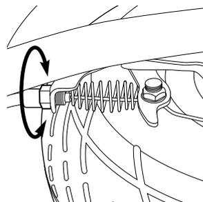
**2 (E125, E200 & E300)** If the brake lever adjuster is threaded outward and the brake still has too much slack, use the rear brake adjuster for additional adjustment.
