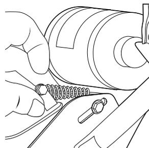
**9** Install the brake spring and thread the cable wire into the cable anchor. Thread the cable to its original position and tighten securely.
