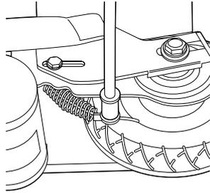
**2** With a 10mm wrench, loosen the brake cable anchor and disconnect the cable.
