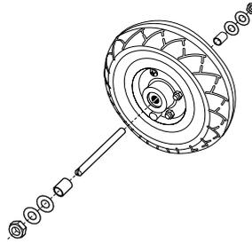
**3** Remove wheel and replace tire. To reinstall wheel, reverse these steps. **Helpful hint:** You may need to use a flathead screwdriver to center the axil and the bolts.
