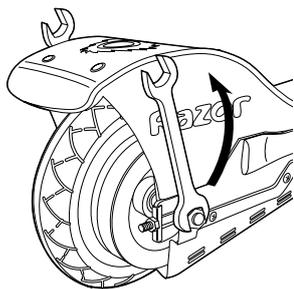
**1** Using two 17mm wrenches, loosen the rear axle bolts by turning the wrenches counter clockwise.
