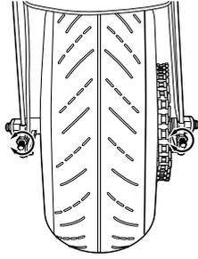
**11** Tighten both axle adjusters the same number of turns to fine-tune the tension on the chain and to approximately maintain the centering of the wheel.
