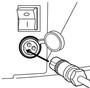
**1** Plug the charger port into the port on the scooter. The charger works with the power switch in either the on or off position. The charging input, on/off switch and overload breaker are located under the deck at the front left-hand side.
