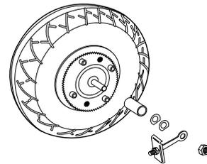
**6** Pull the wheel out. Note the arrangement of the hardware sequence. The spacer order is small, medium and large, with the small spacer between the brake and frame, the medium between the brake and wheel and the long between the wheel and frame.
