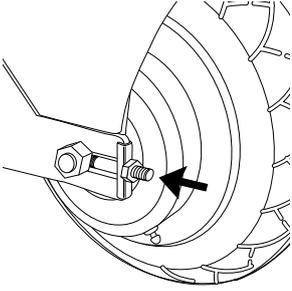
**10** Install the axle adjusters and axle nuts. Tighten until they just barely hold the hardware in place.
