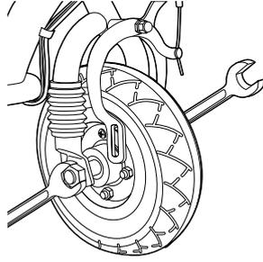
**2** Using two 17mm wrenches, loosen the front axle bolts by turning the wrenches counter clockwise.
