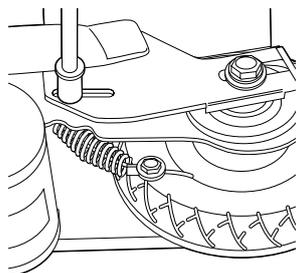
**2** Using two 8mm wrenches, loosen the brake housing anchor which is located in the long slot on the left side of the rear fork.
