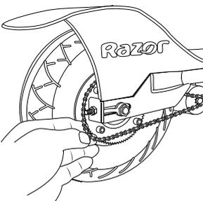
**7** Install new chain or wheel by maneuvering the chain onto the sprocket and slipping the axle into the slots on the frame.
