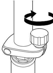
**6** Swing the locking knob to the 12 o'clock position and tighten by hand as firmly as possible.
