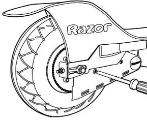
**1** With a Phillips screwdriver, loosen the two screws and remove the chain guard.
