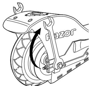
**4** Once the tension is correct, tighten the axle and brake anchor bolt. Test run the scooter. Readjust as needed.
