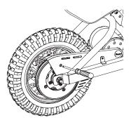
**1** Loosen screw and remove chain guard.
