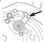
2 If the brake has too much slack, loosen the rear anchor bolt with a 5mm Allen wrench and pull the brake wire tighter. The distance of the brake wire between the end of the cable and the anchor bolt should be between 37mm and 44mm.
