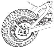
**2** Using two 19mm wrenches, loosen both axle nuts.
