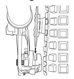
1 Position wheel in front fork and slide disk brake into caliper.
