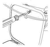
**1** Remove screw from front fork. Align the number plate with the hole in the fork and tighten with a Phillips screwdriver.
