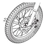
**3** With a 14mm and 17mm open wrench tighten the front wheel screws.
