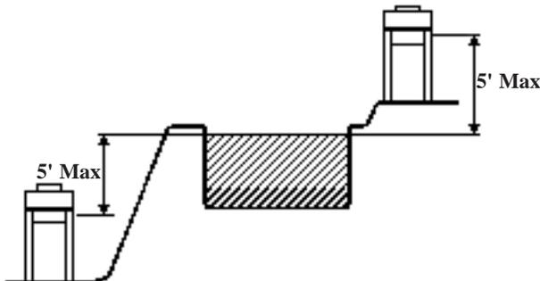
**NOTE:** If heater is installed outside of the limits shown, a flow switch must be used in place of the pressure switch when mounted and wired adjacent to the heater.
