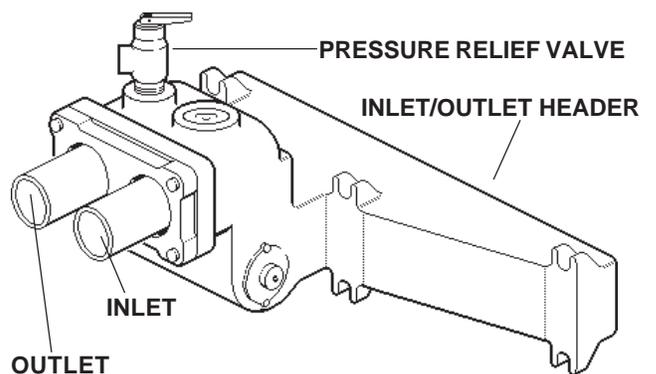
To avoid water damage or scalding due to valve operation, drain pipe must be connected to valve outlet and run to a safe place of discharge. Drain pipe must be the same size as the valve discharge connection throughout its entire length and must pitch downward from the valve. No shutoff valve shall be installed between the relief valve and the drain line. Valve lever should be tripped at least once a year to ensure that waterways are clear.
