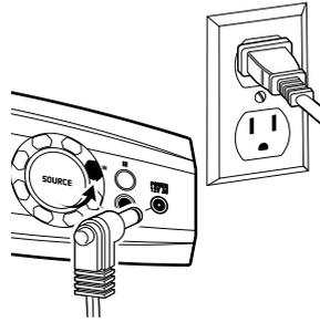
**3** Connect the 12-volt AC power adapter to the electrical outlet and then to the power AC port on the control panel.
