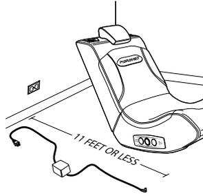
**2** Place the Sound Rocker so that the control panel is less than 11 ft./3.5 meters from the power source.
