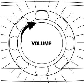
**4** Twist the volume knob on the control panel to click on and test the power. When the power is on all the knobs light up. Twist volume knob to power off the Sound Rocker, then proceed to the connection method shown for your audio/video device.
