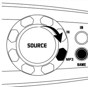
**1** Turn the source knob on the control panel to MP3.
