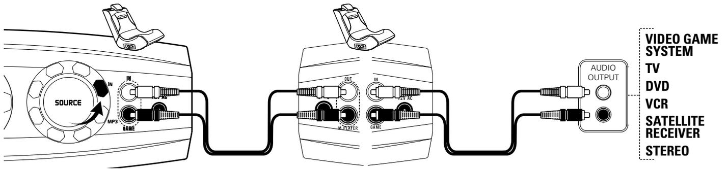
**1** After connecting one Sound Rocker to an audio/video device, you can connect additional Sound Rockers together. Connect the supplied RCA audio cable to the multi-player connection on the first Sound Rocker and then to the input connection on the second Sound Rocker. Repeat to add more Sound Rockers.
