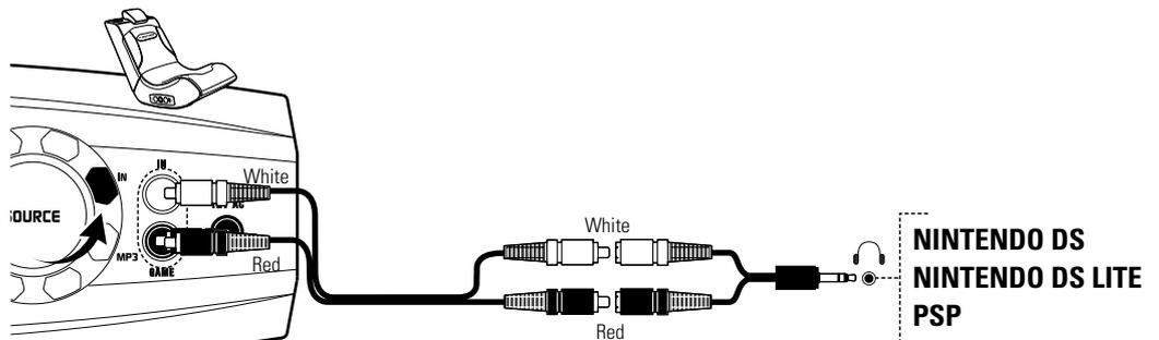
**2** Connect the supplied RCA audio cable from the red and white input jacks on the control panel to the red and white RCA to mini cable and into the headphone jack on your handheld game device.
