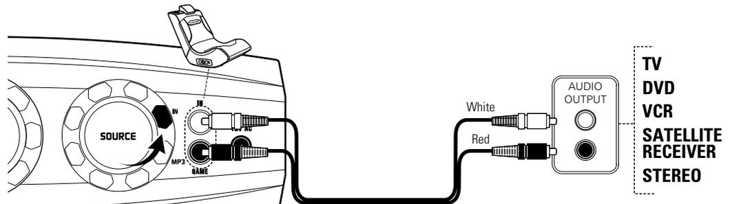
**2** Connect the supplied RCA audio cable from the red and white input jacks on the Sound Rocker to the red and white AUDIO OUTPUT connection on your audio/video device.
