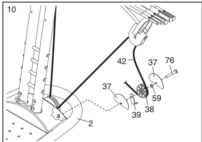
11. Route the Long Cable (42) under a 90mm Pulley (38). Attach the Pulley, a Cable Trap (39), and two Finger Guards (37) to the indicated hole in the Base (2) (see the inset drawing) with an M10 x 47mm Button Screw (76) and an M10 Washer (59). **Make sure that the Cable Trap is oriented to hold the Cable in the groove of the Pulley.**
