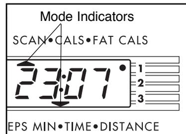
If desired, you can select the reps/min, time, distance, fat calories or calories mode for continuous display. To select one of these modes, repeatedly press the mode button. The mode indicators will show which mode is selected. (Make sure that the scan mode is not selected.)
