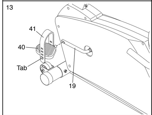
Adjust the Left Pedal Strap (41) to the desired position and press the Pedal Strap onto the tab on the Left Pedal (40). Adjust the Right Pedal Strap (not shown) in the same way.
