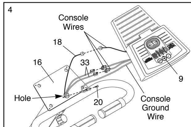
5. Attach the Console (9) to the Handlebar (16) with four Console Back Screws (20). **Make sure that no wires are pinched between the Console and the Handlebar.**
