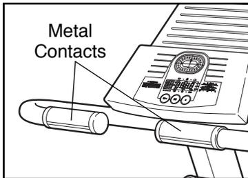
your fingers must be touching the lower contacts. **Avoid moving your hands.** After a moment, the heart-shaped indicator in the display will begin to flash and your heart rate will be shown. For the most accurate heart rate reading, continue to hold the contacts for about 15 seconds.
