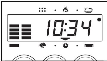
Repeatedly press the mode button until an arrow appears below or above the desired mode symbol. Make sure that there is not an arrow under the scan symbol.
