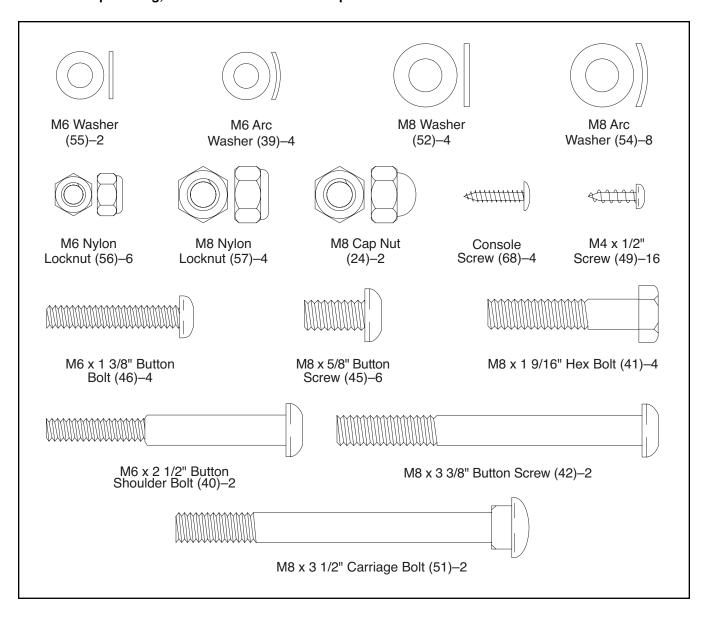
Identify the Front Stabilizer (2), which has Transport Wheels (29) attached to it. Attach the Front Stabilizer to the Frame (1) with two M8 x 3 1/2" Carriage Bolts (51), two M8 Arc Washers (54), and two M8 Cap Nuts (24).
