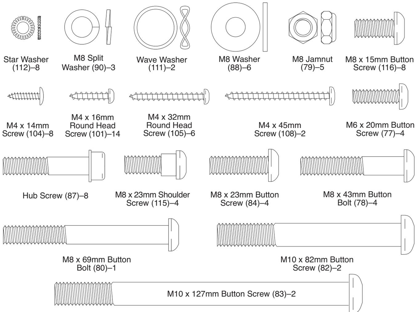
1. While another person lifts the Base (1), attach the Front Stabilizer (6) to the Base with two M10 x 82mm Button Screws (82).
