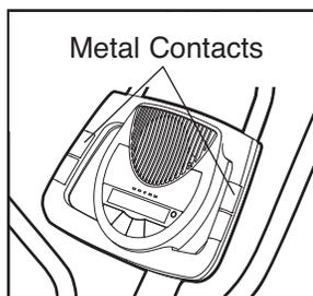
When your pulse is detected, a heart-shaped symbol will flash in the left side of the display each time your heart beats, one or two dashes will appear, and then your heart rate will be shown. For the most accurate heart rate reading, hold the contacts for at least 15 seconds. Note: If you continue to hold the handgrip pulse sensor, the display will show your heart rate for up to 30 seconds. The display will then show your heart rate along with the other modes.
