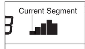
When only three seconds remain in the first segment of the program, both the Current Segment column and the column to the right will flash, a series of tones will sound, and *all target heart rate settings will move one column to the left*. The target heart rate setting for the second segment will then be shown in the flashing Current Segment column.
