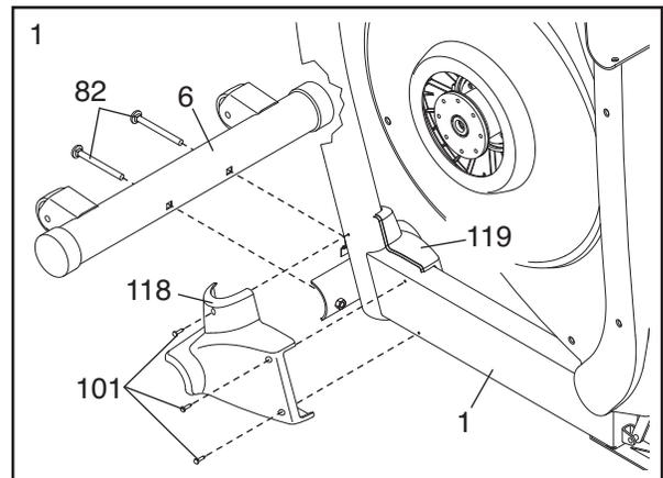
2. Remove the indicated screw and bracket from the Base (1). Discard the screw and the bracket.
