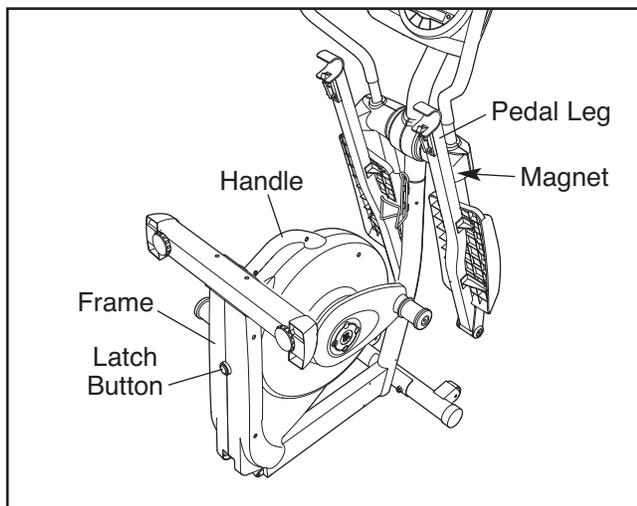
To use the elliptical exerciser, first hold the handle, press the latch button, and lower the frame.
