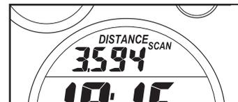
To view only the distance you have pedaled or the number of calories or fat calories you have burned, press the upper button on the left side of the large display until only the word DISTANCE, CALORIES, or FAT CALS appears in the upper section of the large display; make sure that the word SCAN does not appear. To again view the distance you have pedaled and the numbers of calories and fat calories you have burned, press the upper button until the word SCAN reappears.
