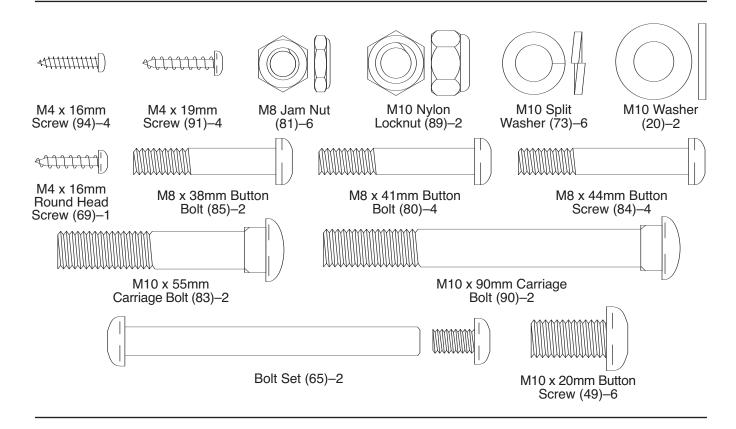
Identify the Front Stabilizer (8). While another person lifts the front of the Frame (1), attach the Front Stabilizer to the Frame with two M10 x 90mm Carriage Bolts (90) and two M10 Nylon Locknuts (89).
