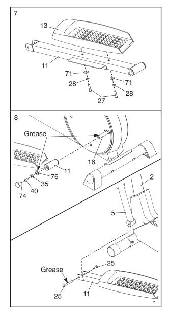
Make sure that all parts of the elliptical exerciser are properly tightened. Note: Some hardware may be left over after assembly is completed. To protect the floor or carpet from damage, place a mat under the elliptical exerciser.
