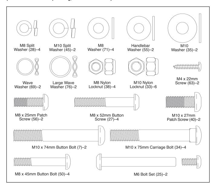
Identify the Stabilizer (9) which has round Endcaps (21) on the ends. While another person lifts the front of the Frame (1), attach the Stabilizer to the Frame with two M10 x 75mm Carriage Bolts (34) and two M10 Nylon Locknuts (33).
