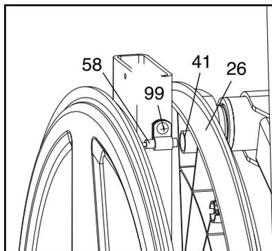
Reed Switch slightly closer to or away from the Magnet, and then retighten the Screw. Rock the Left Pedal Disc forward and backward just enough that the Magnet passes the Reed Switch repeatedly. Repeat
