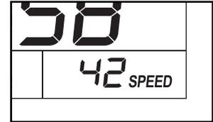
**The upper display**—The upper display is the *priority display*. The priority display can show the elapsed time, the distance that you have pedaled, your pedaling speed, or the approximate number of calories you have burned. Press the Display Mode button repeatedly until the priority display shows the information that you are most interested in viewing. Note: While information is shown in the priority display, the information will not be shown in the lower left or the lower right display.
