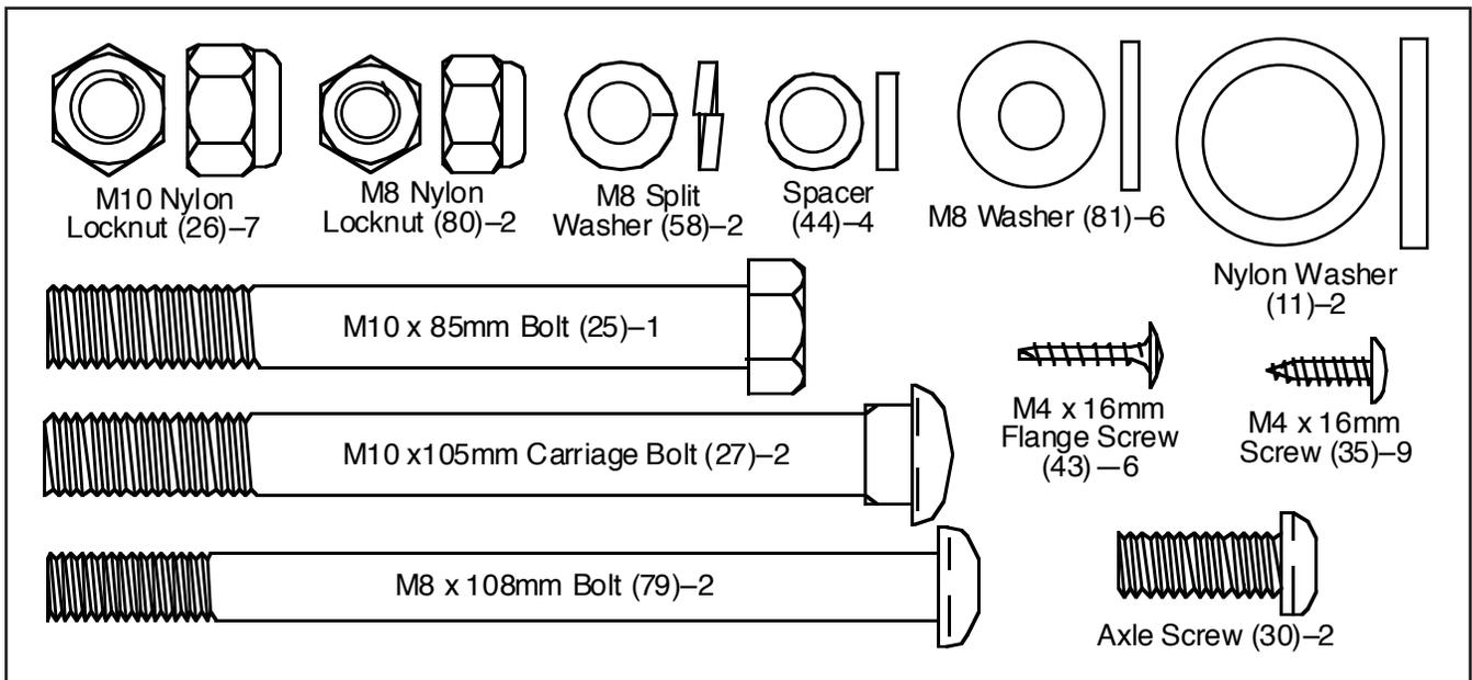
1. Hold the Rear Stabilizer (65) against the saddle on the rear of the Frame (1). Make sure that the Stabilizer is turned so the square holes are facing away from the Frame. Attach the Stabilizer with two M10 x 105mm Carriage Bolts (27) and two M10 Nylon Locknuts (26).
