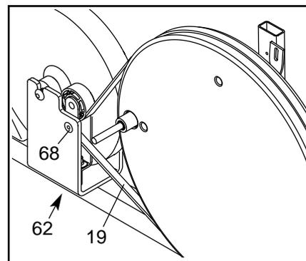
To adjust the Drive Belt, you must first remove both side shields. Refer to HOW TO ADJUST THE REED SWITCH at the left and remove the side shields.
