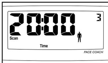
The profiles numbered 1 through 6 on the left side of the console show the resistance and pace settings for the Smart programs. For example, profile number 3 shows that when Smart program 3 is selected, both the resistance and the pace will gradually increase during the first half of the program, and then decrease during the last half.
