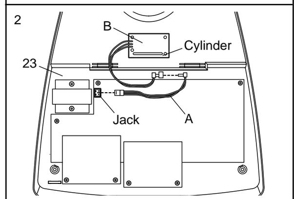
Refer to step 1 above. Reattach the front of the Console (23) with the short and long screws. **Make sure that no wires are pinched.**
