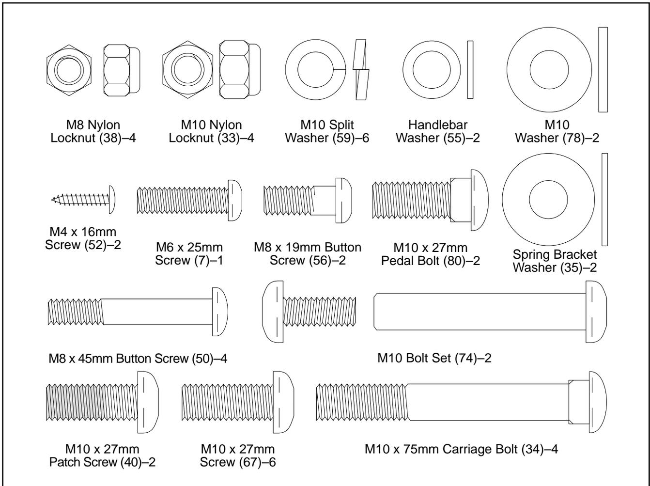
1. Identify the Front Stabilizer (10), which has Wheels (22) attached to it. While another person lifts the front of the Frame (1), attach the Front Stabilizer to the Frame with two M10 x 75mm Carriage Bolts (34) and two M10 Nylon Locknuts (33). **Make sure that the Front Stabilizer is turned so the Wheels are not touching the floor.**
