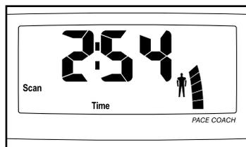
console will show the resistance level for six seconds. In addition, when a Smart program or a Heart Rate program is selected, the display will show the *time remaining* in the program instead of the elapsed time.
