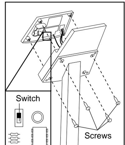
Next, locate the small switch on the back of the console. Slide the switch up or down to change the unit of measurement. Reattach the console with the four screws; **be careful not to pinch any of the wires.**
