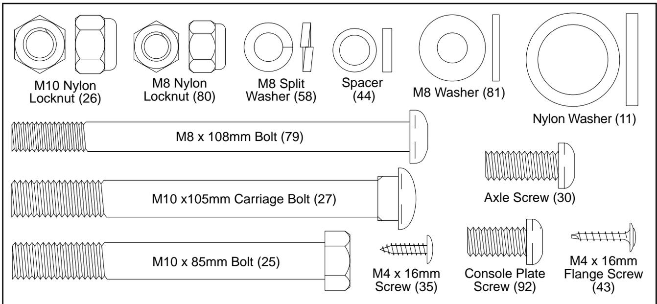
1. Hold the Rear Stabilizer (65) against the saddle on the rear of the Base (1). Make sure that the Stabilizer is turned so the square holes are facing away from the Base. Attach the Stabilizer with two M10 x 105mm Carriage Bolts (27) and two M10 Nylon Locknuts (26).
