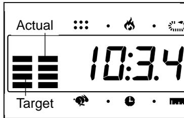
The three graphs on the console show how the target pace will change during the programs. During the Aerobic program (program 2), for example, the target pace will gradually increase during the first half of the program, and gradually decrease during the last half of the program. Each program will last for twenty minutes.
