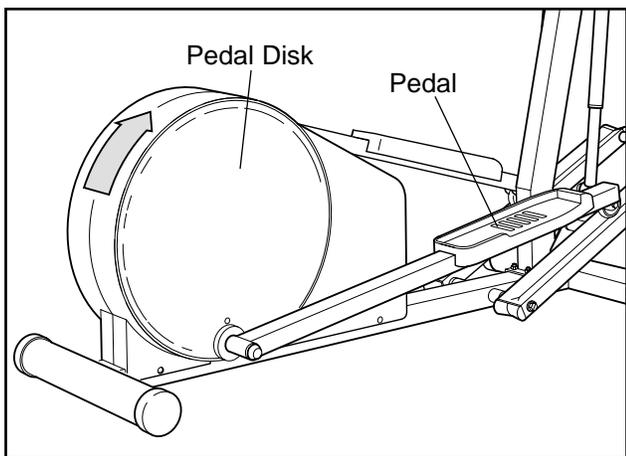
To dismount the elliptical crosstrainer, wait until the pedals come to a complete stop. **Important: The elliptical crosstrainer does not have a free wheel; the pedals will continue to move until the flywheel stops.** When the pedals are stationary, step off the highest pedal first. Then, step off the lowest pedal.
