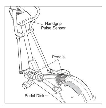
To dismount the elliptical crosstrainer, wait until the pedals come to a complete stop. Note: The elliptical crosstrainer does not have a free wheel; the pedals will continue to move until the flywheel stops. When the pedals are stationary, step off the highest pedal first. Then, step off the lowest pedal.
