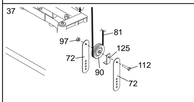
38. Wrap the Lat Cable (81) over a 90mm Pulley (90). Attach the Pulley inside the Rear Top Frame (39) with an M10 x 78mm Bolt (110) and an M10 Nylon Locknut (97).
