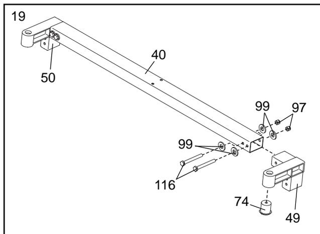
20. Attach the Left Frame Joint (49) to the Left Upright (36) with two M10 x 91mm Bolts (116), four M10 Washers (99), and two M10 Nylon Locknuts (97). **Do not tighten the Locknuts yet.**
