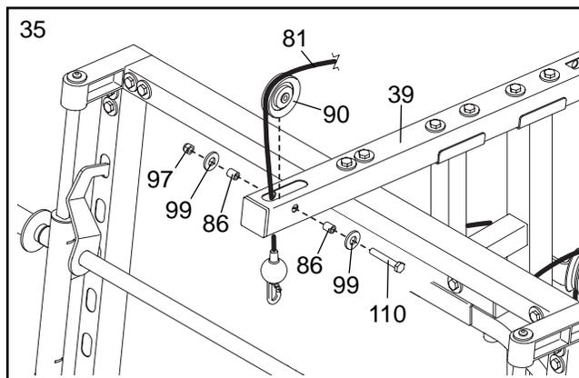
36. Route the Lat Cable (81) over a 90mm Pulley (90) and down through the Rear Top Frame (39). Attach the Pulley inside the Rear Top Frame with an M10 x 78mm Bolt (110), two M10 Washers (99), two 17mm Spacers (86), and an M10 Nylon Locknut (97).
