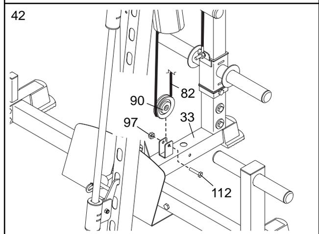
43. Route the Low Cable (82) over a 90mm Pulley (90) as shown. Attach the Pulley and a Cable Trap (125) to the second set of holes from the bottom of the two Pulley Plates (72) with an M10 x 45mm Bolt (112) and an M10 Nylon Locknut (97). **Make sure the Cable Trap is oriented to hold the Cable in the groove of the Pulley.**
