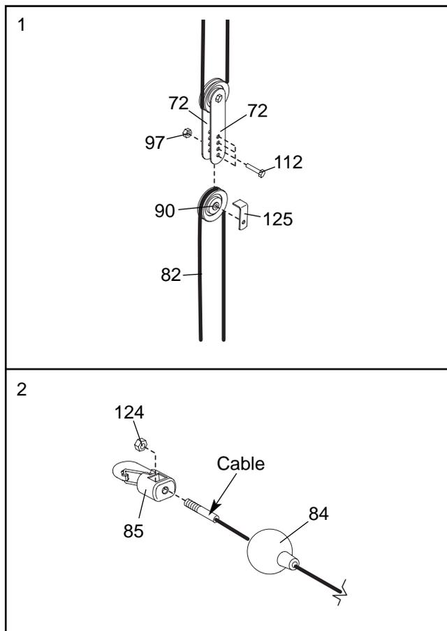
**See drawing 2.** Additional slack can be removed from the cables by tightening a cable into the M6 Nylon Locknut (124) inside a Cable End Clip (85). To do this, pull the Clip Cover (84) back and use pliers to tighten the Locknut. Replace the Cover.
