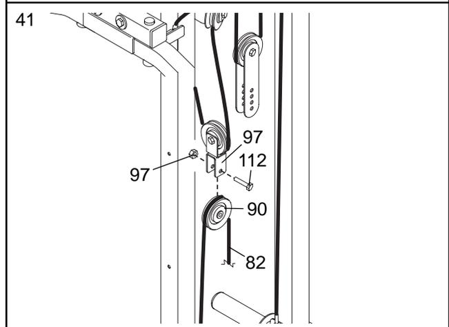
42. Route the Low Cable (82) under a 90mm Pulley (90) as shown. Attach the Pulley to the Rear Base (33) with an M10 x 45mm Bolt (112) and an M10 Nylon Locknut (97).
